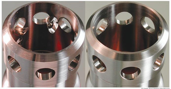
Heule cutting tools, along with BRM's Flex-Hone tools, remove burrs and caps created when drilling holes in nickel, Inconel, Waspalloy, titanium and stainless steels. A precise, smooth though-hole is critical for aerospace parts.
