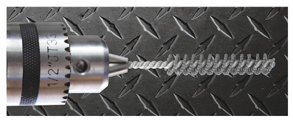
In combination with Heule cutting tools, a major jet engine component manufacturer applies the Flex-Hone from Brush Research Manufacturing on the machining center for final deburring of through-holes, which is usually an expensive and time-consuming manual operation.
