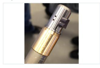
The proposed solution from HEULE is the countersinking tool SOLO.
