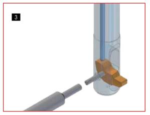
**Assembling** - Insert the blade. Then insert the split pin and fix the blade.
