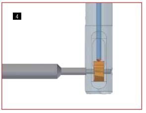
With the flat side of the assembly pin, push in the split pin until it is flush with the blade housing diameter. Blade is fixed in place.
