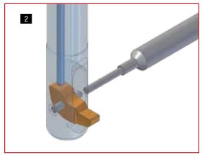
Position the assembly pin on the solid end of the split pin (opposite side of the slot). Press the assembly pin in until the split pin falls out and the blade is free.
