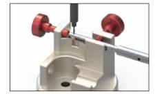
Push the split pin carefully out of the bore. Make sure you apply the assembly pin to the split end of the pin. If necessary, use a small hammer.
