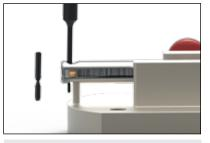
Insert new roll pin short section first into the hole until the back end of the pin is flush with tool holder.
