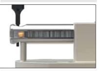
In order to define the right position of the blade and to pre-center for the new roll pin, push the assembly pin in the roll pin hole.
