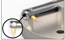
Insert new blade with cutting edge up into the blade holder. Make sure that the blade is pushed in from the line mark side.
