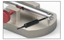
Use the assembly pin to make sure the blade hole and the pin hole are aligned. Press the assembly pin all the way through to the larger diameter.
