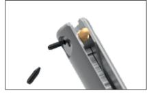
Loosen clamping screw and take the tool into your hands. Manually brake off the projecting section of the roll pin at the predetermined breaking point.
