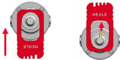
To CHECK the Tool Function (extension and retraction of the blade) insert the SOLO Key and turn clockwise. The Blade should move out. After the Blade function test, re-position the Housing until the position pin hits the end stop. The Housing position mark must line up with the notch mark on the Tool Head.
