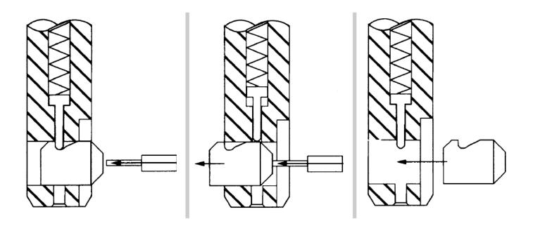
Please note: Blade can be installed from either side of the tool.
