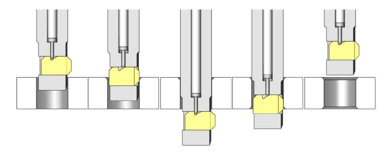
As the rotating tool is fed into the hole, the front cutting edge deburrs the top of the hole by cutting a 45° chamfer. As the tool feeds into the part the blade is forced into the body and slides in the blade window.
